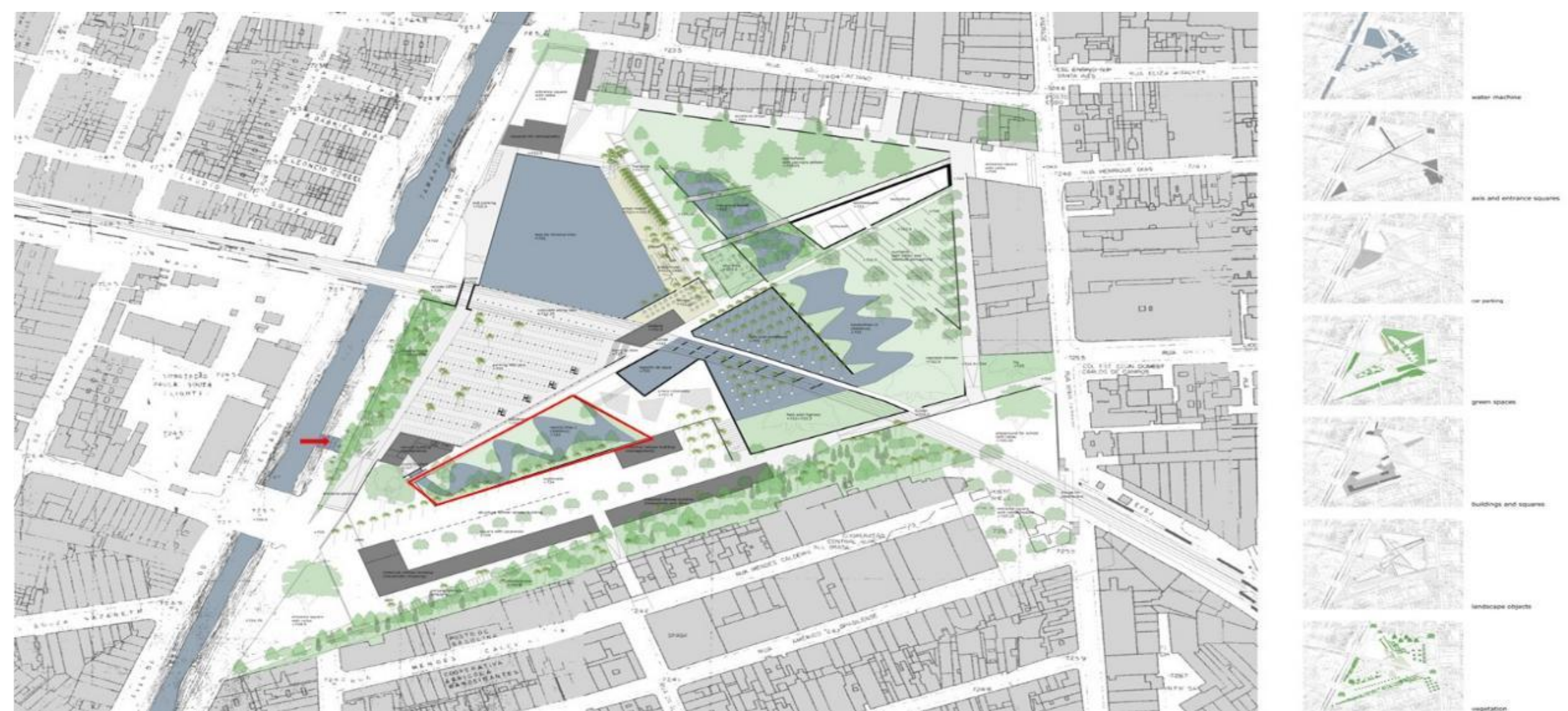
A helophyte filter in a park near Rio Tietê in Sao Paulo Brasil. The red arrow is the inlet towards the helophyte filter. The red outlined area is the helophyte filter of Typha domingensis as applied in a winding water system to enlarge the interaction between cattail and the purification of inlet water. The water purification passes several other plant filter systems and end in a recreational pool of swimming water quality and overflows back into the Rio Tietê (Source: drawing by Ir. Sander Troost, 2009)
